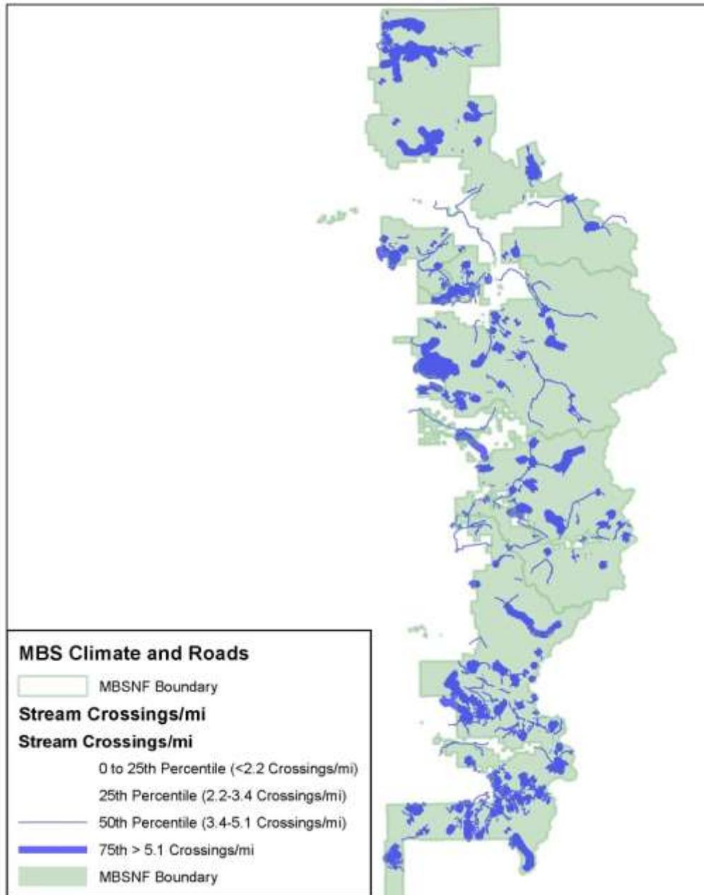
Figure 8. Stream crossings per mile of road. Roads with > 5.1 stream crossings per mile (75<sup>th</sup> percentile) are shown in heavy blue. Roads below the 50<sup>th</sup> percentile of crossings per mile are not shown.
