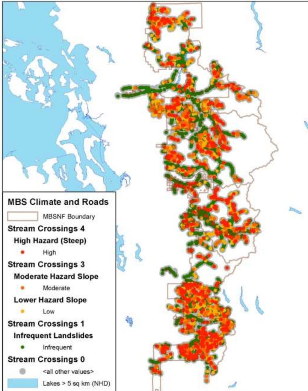
Figure 7. Road-stream crossings on the MBSNF. The hazard ranks were determined based on slope as explained in the section on hazardous stream crossings.
