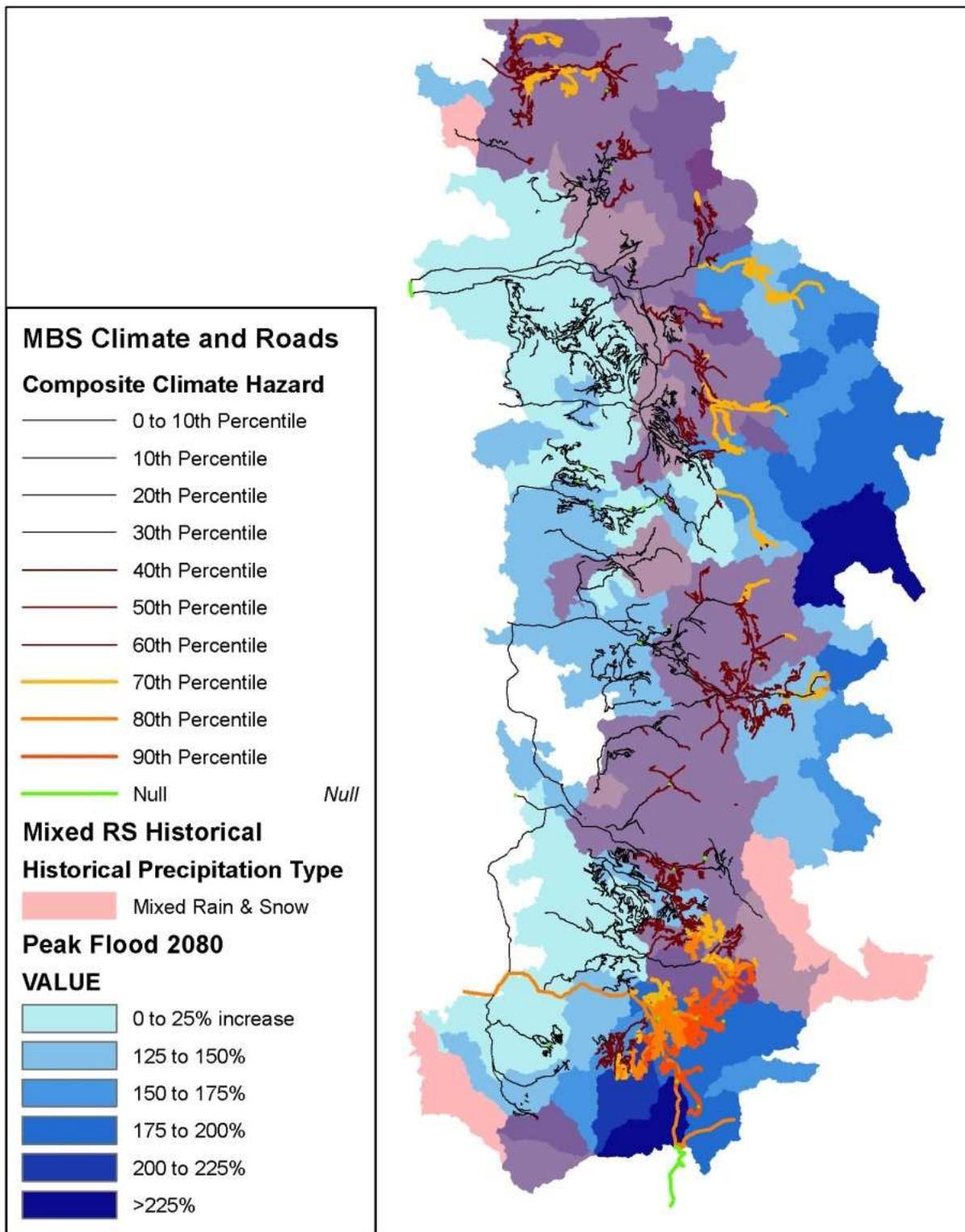
Figure 2. Composite road hazard scores overlaid on the potential 2080 peak flood level percent increase for each subwatershed, with mixed rain-and-snow subwatersheds shaded darker.
